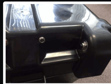
• A 2.5mm DC power jack must be fitted. A Plastic Jack is preferred. • A 10A automotive style circuit breaker must be fitted
